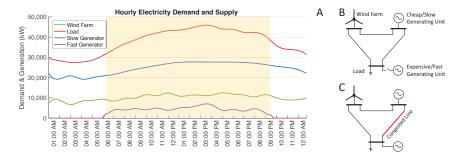
FIGURE 1. Day-ahead scheduling of a notional power system, with three vertices and two generating units. (A) The optimal operational strategy based on the available forecast of the demand and wind generation. The shaded period represents peak hours. (B) Off-peak configuration of the network, during which the expensive generator is not committed. (C) Peak configuration, during which the expensive generator contributes to accommodate transmission limits.
